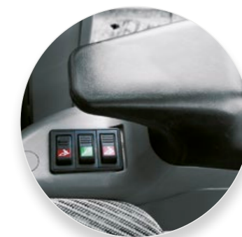
Lockable push button for actuation, protected against accidental unlocking. Locking control via indicator pin on quickcoupler
