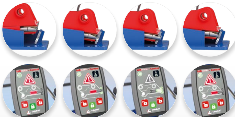
Quickcoupler unlocked, not yet fully in adapter
